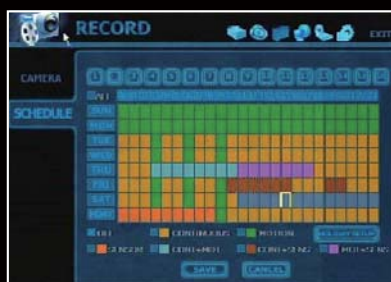
Various recording modes by channel, date, and hour in different colors
